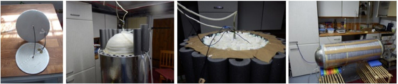
Figure 3: Heating foil under the earth-plate; Thermal insulation upper dome and sidewall; Hoses for Thermostats
